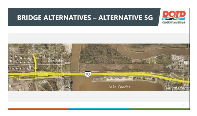
Alternative 5G was designed to provide a compact and complete interchange at Sampson Street. It does not require an extension of Sulphur Avenue because Sampson Street will be raised to connect to the bridge above grade, eliminating all conflicts with the railroad crossings on Sampson Street.
