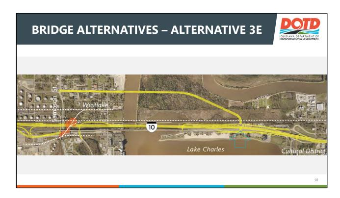
Alternative 3E differs from Alternative 3A only in that the interchange at North Lakeshore is complete (1). That is, drivers can enter or exit the interstate from all directions by way of the Sulphur Avenue extension. But they may also use I-10 to cross the river entering or exiting at Sampson Street. All other operational and access features, including the long-span crossing of the EDC (2), are the same as 3A.
